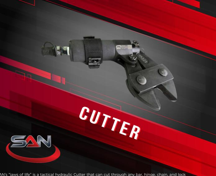
SAN's "jaws of life" is a tactical hydraulic Cutter that can cut through any bar, hinge, chain, and lock with a cutting force of 22.4 tons. At the blades' junction, tactical operators can cut through elements with diameter up to 18mm. Thanks to its innovative design the element can be cut without any risk of slipping during the operation and the Cutter enables the operator high accuracy and safety capabilities.
